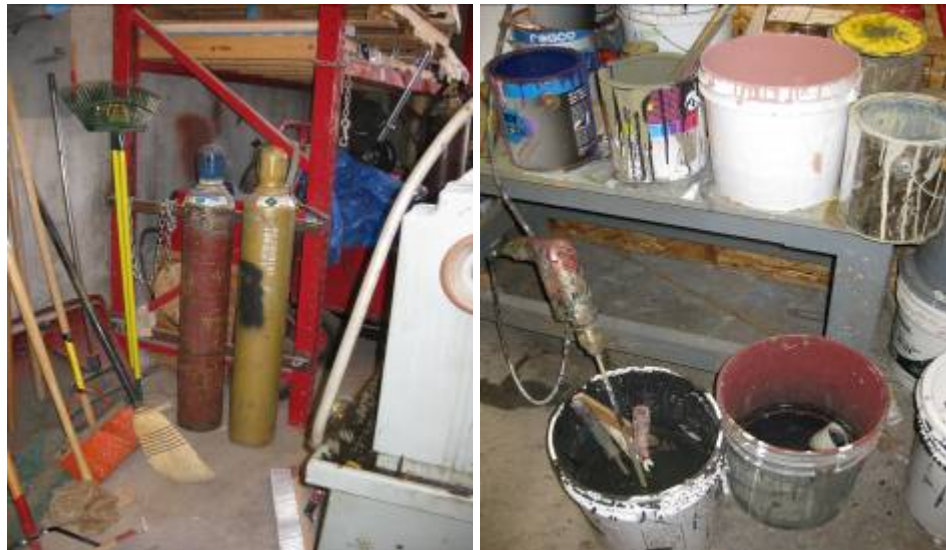
Unchained compressed gas cylinders.
